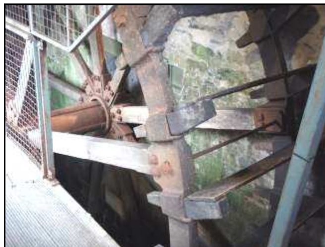
Figure 16 – Corn Mill breast shot waterwheel. Cast iron and wood with flat paddles.
